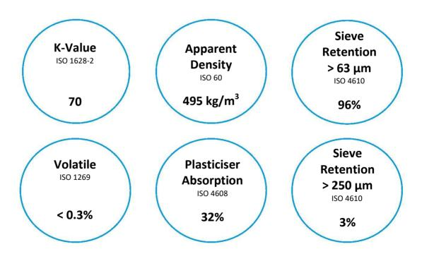
Note: The property data shown above has been obtained from laboratory tests on representative samples of VYNOVA<sup>TM</sup> S7102 polymer. Although the values are typical, they are for guidance only, and must not be used as a basis for specifications.
