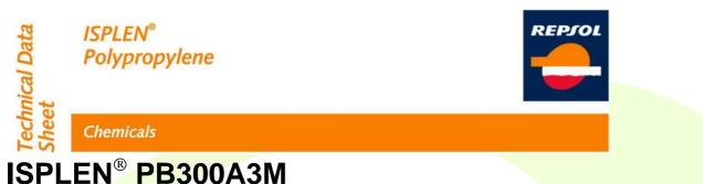
ISPLEN<sup>®</sup> PB 300 A3M is a very high fluidity heterophasic copolymer characterised by its excellent flow properties and good balance of mechanical properties, impact strength and high stiffness. It is particularly suitable for injection moulding applications used in the manufacture of very thin walled articles.
