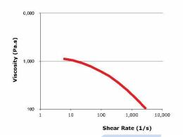
The above values were Calculated from data for 100 µm produced on a 75mm Barrnage extruder with 190°C melt temperature using a 2:1 blow ratio and a gap die of 3.0 mm.
